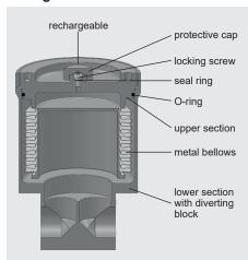
Example design of a metal bellows accumulator with diaphragm bellows
