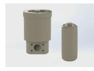
Accumulator type: SM50P and SM50 Nominal volume: 3.8 and 1.6 litres Material: Carbon steel, coated Version: Corrugated bellows
